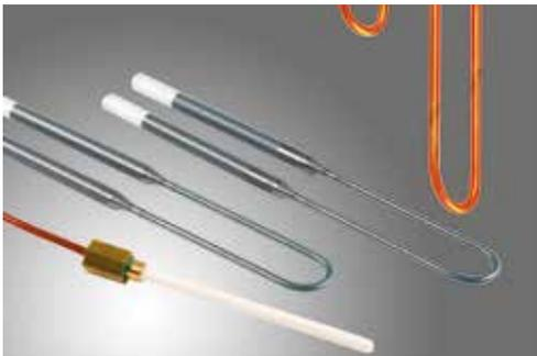
High-quality molybdenum disilicide heating elements reach a maximum end temperature of 1.650°C. Unlike silicon carbide heating systems, heaters of this type are far enough away from their maximum performance limit of approx. 1.800°C. Thanks to this property they attain a significantly longer service life. Each of the four heating elements can be individually replaced in case of damage – an „en bloc“ replacement is unnecessary.
